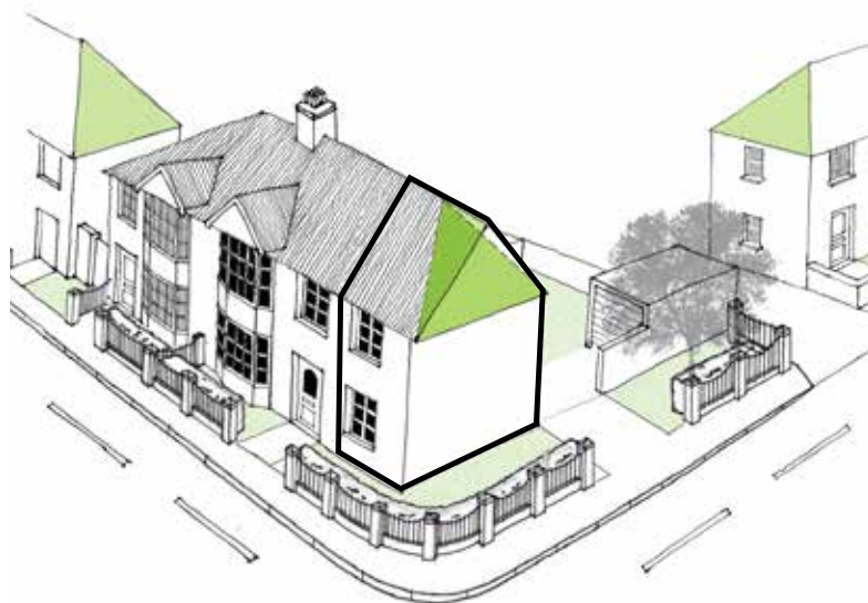
A hip-to gable extension with no regards to the existing hipped roof profile of its streets.
